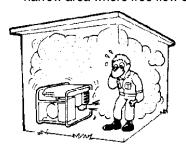
flow is restricted it will cause serious damage to the generator or engine and may cause injury to people. Remember the generator engine gives off DEADLY carbon monoxide gas.
